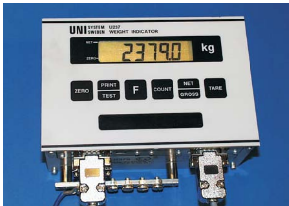
Picture shows 230VAC-power, indicator and table scale.
